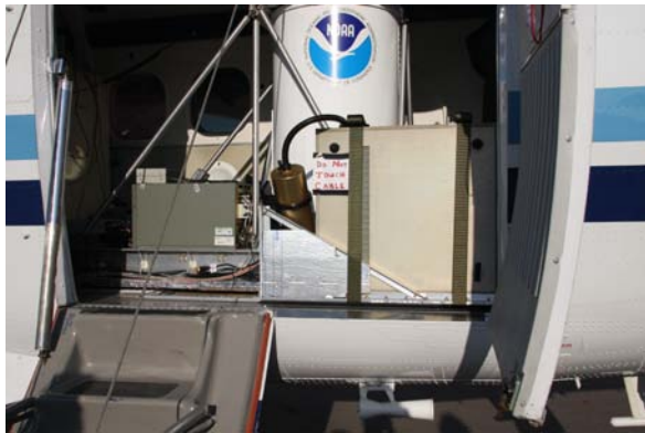
Figure 2. Photo of the Salford Halo lidar as installed in the Twin Otter. The lidar includes a control unit (rectangular box with straps) plus a laser head (cylinder with umbilical). The TOPAZ lidar telescope, positioned directly over the nadir port, can be seen behind the Salford lidar.
